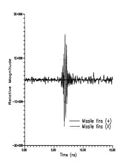
Figure 5. Cross-polarized scattered field response of isolated missile.
