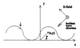
Figure 1. Geometry for finite sized 2-dimensional conducting surface.
