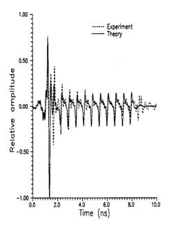
Figure 2. Comparison of scattering from sea surface model for TE polarization.
