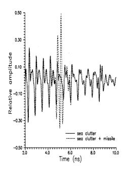
Figure 3. Scattered field response of 2" missile model over sea surface for TE polarization.
