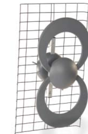
LOOP DE LOOP: The new ClearStream2, from Antennas Direct, uses thicker-than-traditional elements and tapers the thickness of the loops, which allows the antenna to respond to a greater range of frequencies. The resulting tapered-loop antenna is half the volume of the equivalently performing bow-tie array that has been on the market for years. As with the SquareShooter, the grid acts to defend the antenna against multipath interference.
