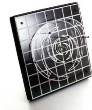
UNDER THE HOOD: The Winegard SquareShooter consists of a two-arm sinuous element and grid reflector attached to an inexpensive Mylar substrate and encased in a plastic dome. The element responds across a broad range of frequencies; its size is optimal for the UHF band. The open grid behind it is sized to reflect UHF frequencies, which reduces the multipath problem by blocking some of the signals that bounce off buildings or hills instead of coming directly to the antenna.
